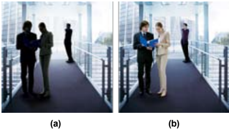
Figure 2.13 Image quality (a) without WDR and (b) with WDR
