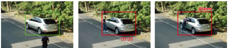
Figure 10.6 Alarm triggered by loitering detection
